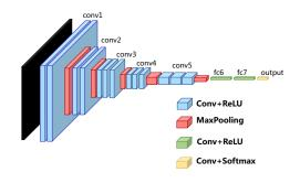
Figure 4: VGG-Face architecture
